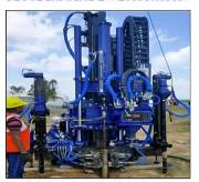
Geotechnical Investigation by rotary and/or wireline Drilling in all Types of Soil & Rock using TMG multipurpose drilling rig (imported from USA, fully automated SPT with Energy Measurement, SCPT, in situ vane), preparation of Engineering reports, including Liquefaction Assessment for both onland and offshore projects.
